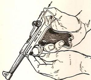
2. Cock the pistol by pulling the rear toggle link upwards.
