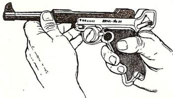
7. To reassemble, slide in barrel and receiver on the frame.
